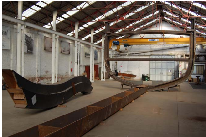
The new shipbuilding hall at Boom with full scale keel and hull sections of the Belgica replica.
